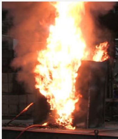
Large-scale free burn of LFP batteries after 71 minutes
